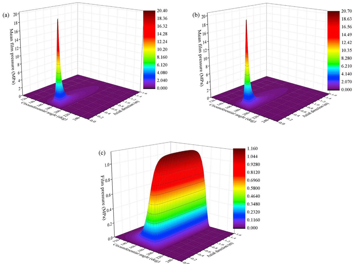
**Fig. 4.** Mean hydrodynamic pressure distribution at rotational speed of 160 r/min: (a) Considering turbulence and journal misalignment; (b) Considering journal misalignment without turbulence; (c) Not considering journal misalignment and turbulence.
