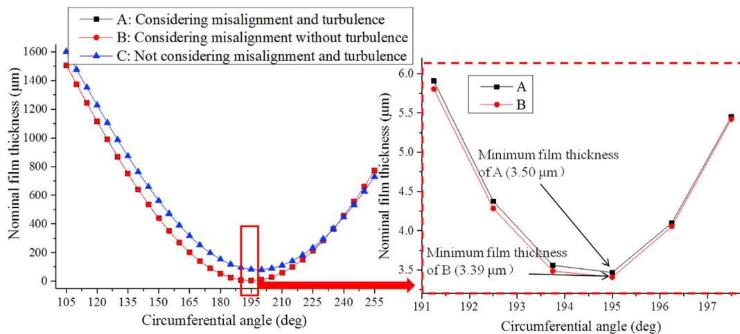
Fig. 6. Nominal film thickness distribution at the rotational speed of 160 r/min.
