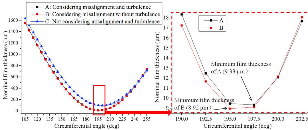
Fig. 7. Nominal film thickness distribution at the rotational speed of 190 r/min.
