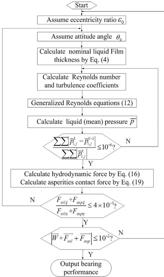
Fig. 3. The flow chart of numerical calculation.
