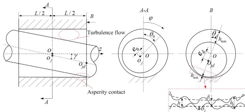
Fig. 1. Geometry model of the misaligned journal bearing.
